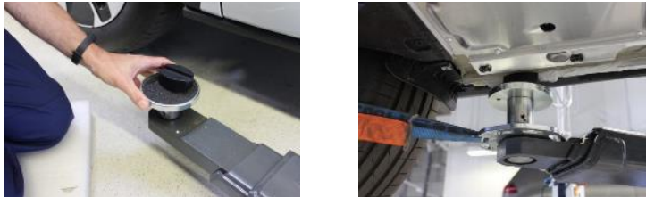
The ATS support plate system with form-fit vehicle adapters in use Photos: MAHA
