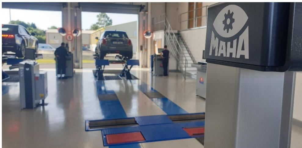
MAHA's DUO scissor lifts in use at Vehicle Inspection Centres Photo: MAHA Ireland
