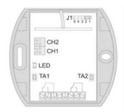
Mode of operation:Dead man's control (each<br/>relay switches as long as<br/>the corresponding button<br/>is pressed (max. 36s)Setting:Jumper J1 in position 1-2Antenna:Antenna is located inside<br/>the control cabinet,<br/>therefore a direct line of<br/>sight from the vehicle to<br/>the control cabinet is
