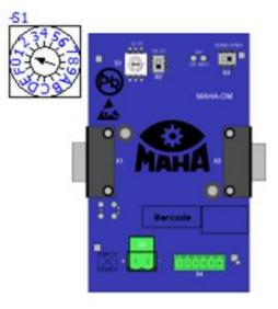
Address (CAN ID) of the OM: **S1:** 0-15, if **S2** is set to 0 (down) **S1:** 16-31, when **S2** is set to 1 (up) **S3**: Term only on the last module **Setting according to specification as per circuit diagram**
