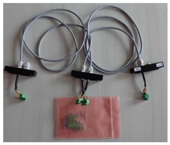
The GSQ sensor elements must always be mounted in pairs (GSQ sensor transmitter with opposite GSQ sensor receiver) in the pit. The addresses of the GSQ sensor elements must always be set to the same value with its opposite transmitter/receiver by means of the **S3** rotary switch. Starting with the address 1, the address is increased by one with each following sensor pair.
