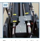
The stroke travel of both cylinder pairs on each scissor side is measured via cable pull potentiometer, the hydraulic synchronization is conducted automatically by the control. The operator is freed from manual leveling compensation.
