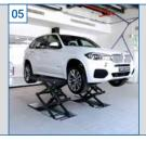
Flush-floor routing of hydraulic hoses and cables possible, no tripping obstacles for persons!
