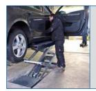
The vehicle doors of the lifted vehicle can be completely opened. The free side access to the vehicle offers comfortable working conditions.
